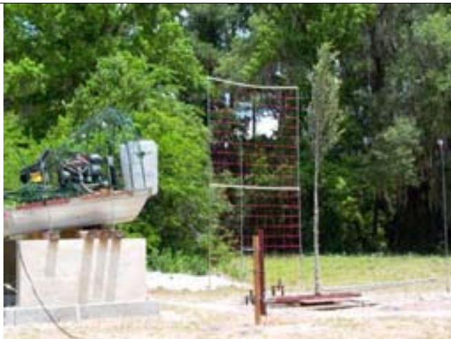
Airboat generated up to 70 mph winds blowing against the canopy of Highrise® live oaks
