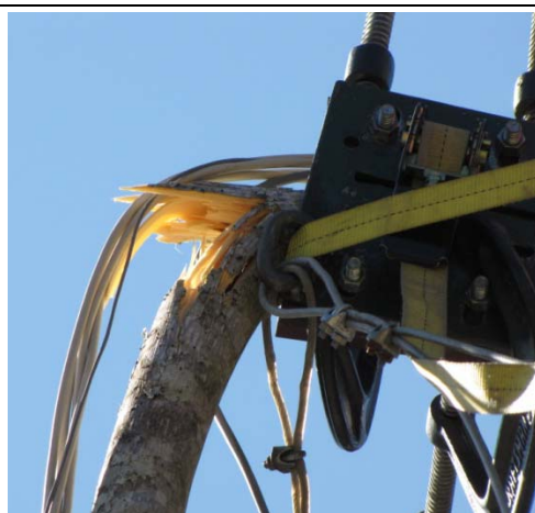
Horizontally oriented branches typically failed within the first several inches from the branch base.
