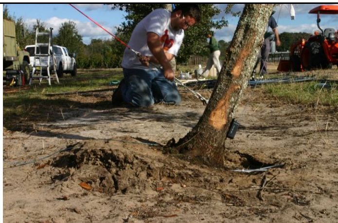
Root ball sat tilted after pulling trunk to 25 degree angle. The leeward side of the root ball sank (see right side of trunk) at the point where the original #15 container was; the windward side broke from the ground at the outer edge of the #45 container (see left side of photo).
