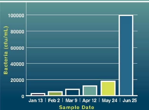
**I**N this holding tank, which contained water directly from the well, a rise in overall bacteria counts (and fungi, not shown) over time was an indicator that the copper system was not adequately controlling biological load. Corroded electrodes in the copper system were the culprit. It is important to note that no bacterial or fungal disease was evident on crops in this or the other greenhouses in our study despite some high colony counts.
