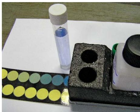
**On-site tests allow growers to check the concentration of control agents. Sample on-site test kits for a copper treatment system (left) and ZeroTol (right).**
