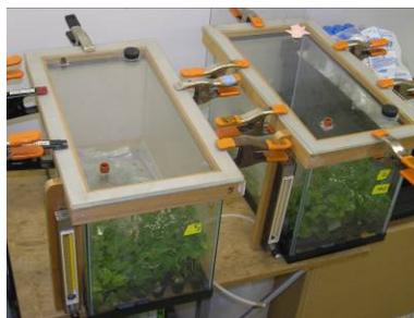
**Figure 2 Glass tanks sealed with metal clamps with unrooted cuttings (bags) and liners.**
