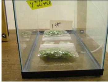
**Figure 4 Tank with two bags of cuttings and two EthylBloc sachets**
