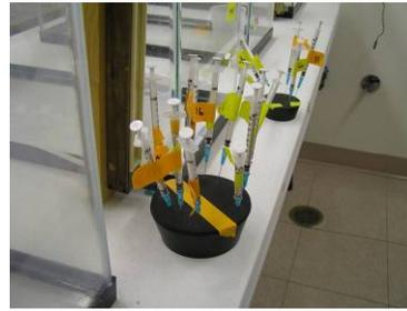
Syringes used to measure ethylene levels
