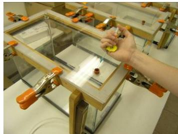
Measuring 1-MCP levels inside tanks
