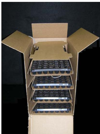
Uninsulated Box with trays and temperature sensors.
