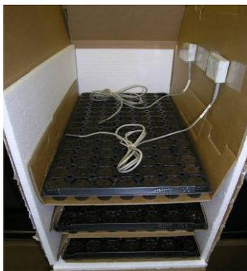
Photo demonstrating how sensors were taped to the top of the third cardboard insert. Leads were fed out through the corner of the box.
