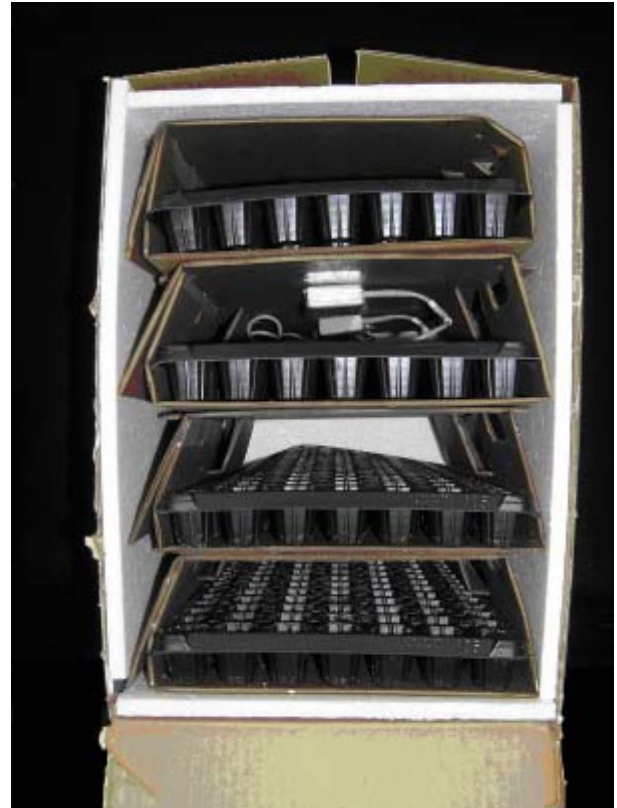
Cross section of an insulated box with all four trays, temperature sensors and media.
