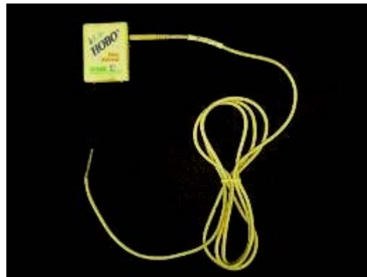
HOBO Temperature sensor and external lead used in experiment.
