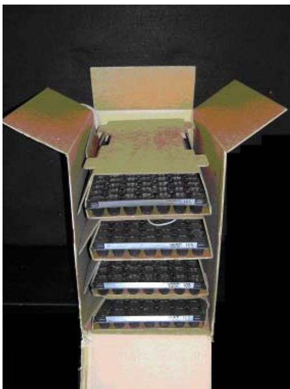
Uninsulated Box with trays And temperature sensors.
