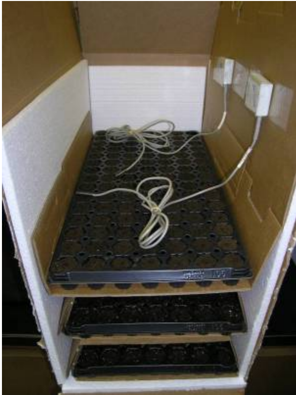
Photo demonstrating how sensors were taped to the top of the third cardboard insert. Leads were fed out through the corner of the box.
