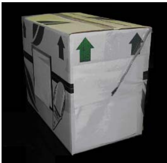
Photo of closed box with external leads taped to outside.
