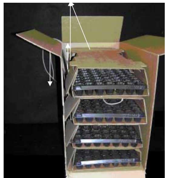
Another photo (uninsulated box this time) illustrating how leads were pulled out of box.
