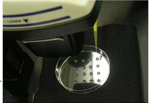
Viability test. Photo shows the 40 $\mu\text{L}$  droplets being applied to the petri dish and then viewed through a dissecting scope to count the number of active and inactive EPN.
