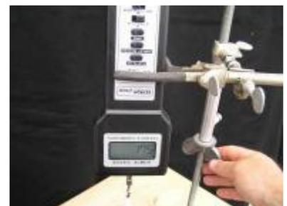
The tension meter was set to record the peak tension require to pop the plug out of the tray.
