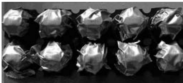
Figure 5. To measure media air porosity, the drainage holes of plug cells were covered with tapes and slowly adding water to the medium until reaching saturation point. The cells were weighed when the drainage hole was covered (plugged), then unplugged, drained and weighed again.
