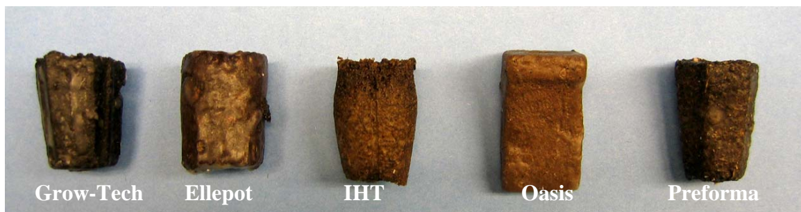
Figure 3. To calculate the volume of the simple stabilized media, media were first moistened then coated with paraffin. The volume of each type media was then estimated by water displacement.
