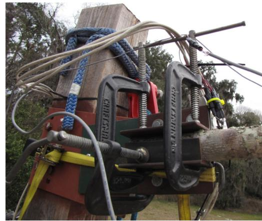
Fig. 1. Branch mounting bracket and branch secured to vertical post.
